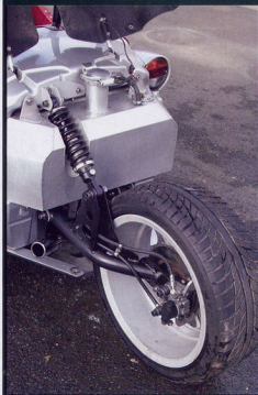
Front uses VW Golf uprights and fabricated wishbones. Has an anti-roll bar, too.
