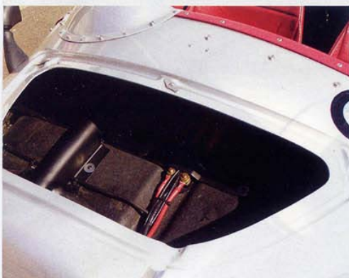
Luggage space is enhanced by the front locker under the scuttle. Interior panels can be removed to gain access to the pedal box and the rear of the dashboard.
